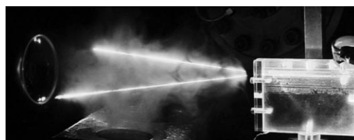
Figure 13. Optical PEFC with two laser beams focused to a point within the flow channel.
