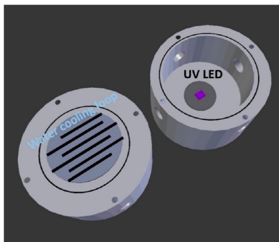
Figure 14. Schematic diagram of the Gen-1 photoresponsive membrane test cell. Reprinted with permission from ref 91. Copyright 2018 Springer Nature.
