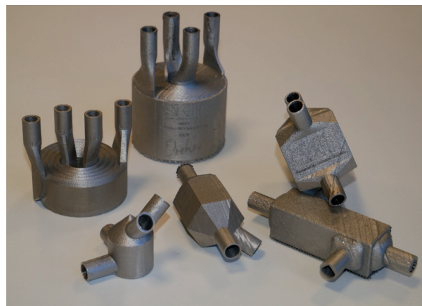
Figure 9. Different printed heat exchangers from the course. They clearly show the motivation and creativity of the participants.
