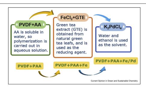
An example of green synthesis of membranes using natural available resources. AA, acrylic acid; PVDF, polyvinylidene fluoride.
